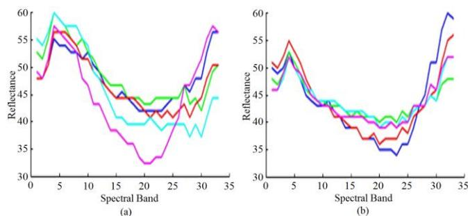
Fig. 3. Spectral responses of (a) each blue ink type and (b) each black ink, showing that blue inks are easily distinguishable as compared to the black inks in the UWA WIHSI database.
