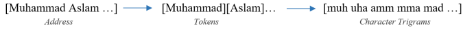
Fig. 2. Flow of division of address into tokens and tokens in to character trigrams.
