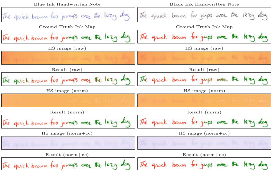
Fig. 10. An illustration of ink mismatch detection on a blue ink and a black ink handwritten notes, acquired using adaptive exposure. The ground truth ink pixels are labeled in pseudo colors (red: ink 1, green: ink 2). The spatially non-uniform illumination pattern can be observed in raw HS images, with high energy in the center and low towards the edges. Normalization removes the illumination bias and greatly improves segmentation accuracy. Color constancy improves the visualization of HS images, while resulting in comparable accuracy.
