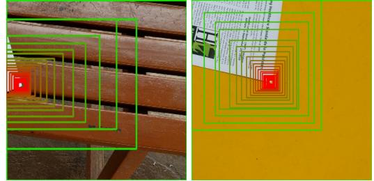
Fig. 4: Recursive Corner Refinement. Based on prediction the area least likely to contain the point is discarded and cropped image is fed to the model again. The squares represent the area that the model sees in each iteration.
