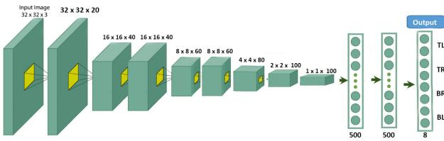
Fig. 3: Model architecture for corner detection. 5x5 kernels are used and Rectified Linear Unit (ReLU) is applied after every convolutional layer. The eight outputs are interpreted as co-ordinates of four corners.
