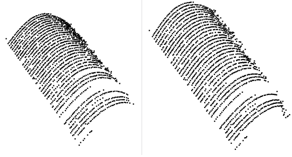
Figure 1: 3D reconstruction of book page. Left side shows results after application of RANSAC. Right side shows original output.
