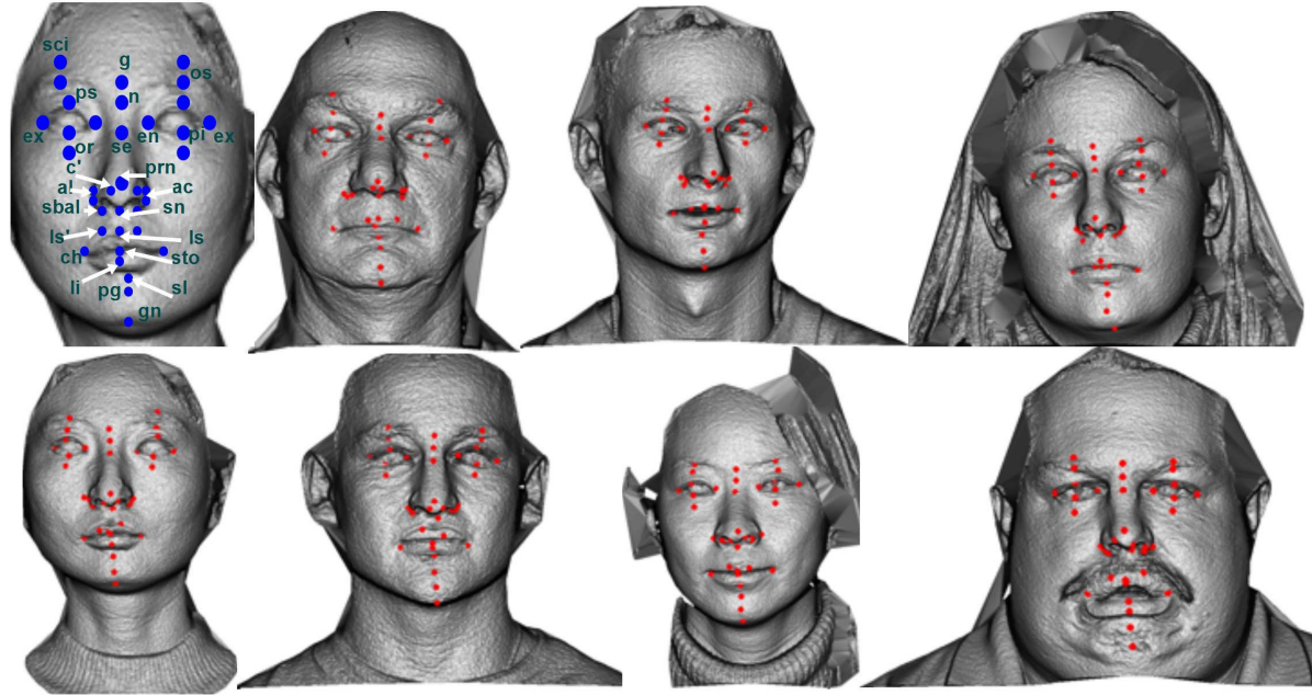
Figure 9. Thirty five anthropometric landmarks [15] automatically detected on seven identities of the FRGCv2 database. The top left face gives the ground truth locations and names of these landmarks. Notice, the consistency and accuracy of detection.
