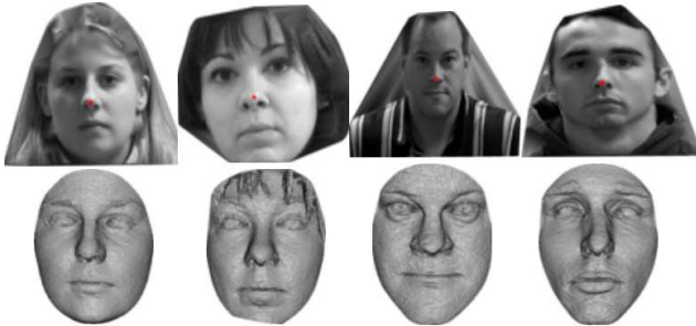
Figure 3. Preprocessing shown on four identities of FRGCv2 database. The upper row corresponds to the raw 3D image with texture while the lower one is the output of our preprocessing step.
