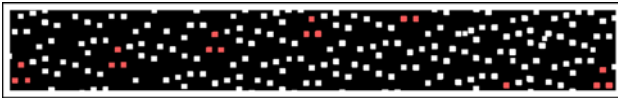
Fig. 12 Example of a diffuse pattern. It can be seen that the pattern is repeating in horizontal direction but that the repetitions have a small offset. A characteristic set of dots is colored in red to make the repetitions more easily detectable (color figure online)
