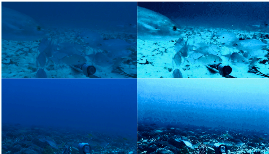
Fig. 6. Image enhancement: First column are raw images. Second column shows enhanced images as a result of histogram equalization.
